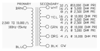
your job is to determine which wire goes to your positive signal lead on your output jack. You are going to install a resistor between this wire and the jack. If you are using 8 ohms impedance, it will be a yellow wire. You can use a meter to verify which wire is the signal wire. You should read a short between that wire and point "A".
