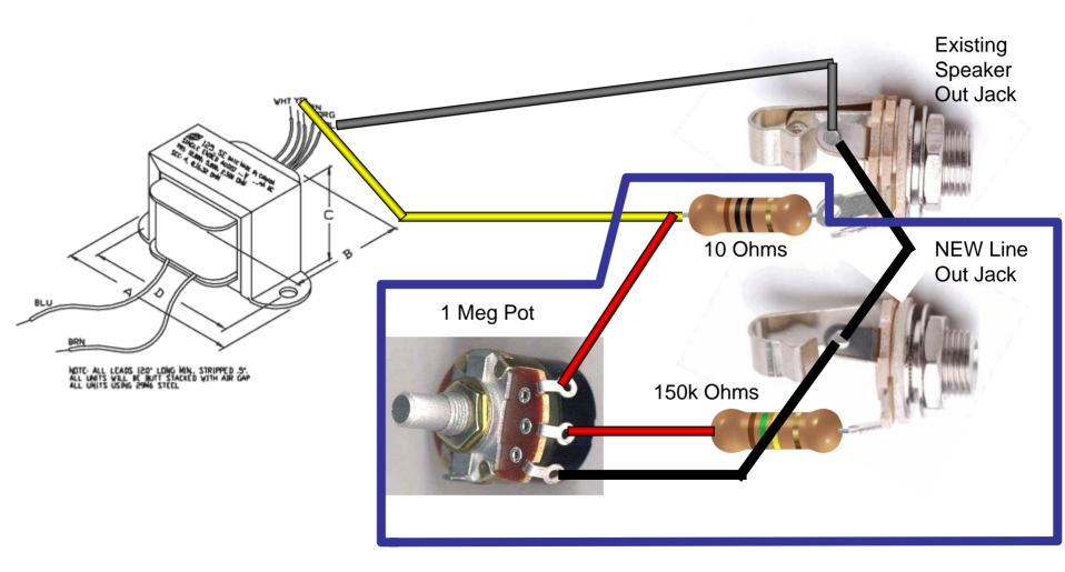
All the stuff in the blue box is new. Note the black wire is your ground path. It attaches to the ground side of the level pot, then ground on your new line out jack, AND then attaches to the old ground tab on your speaker jack.
